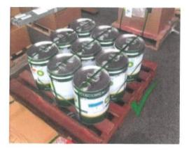
• Steel drums are to be strapped together with steel strapping
