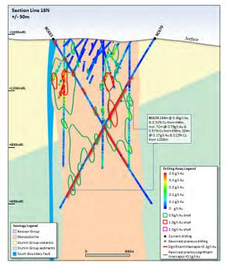
**Figure 21.** Schematic cross section of RC665 and RC670 showing Newcrest and Imperial drill holes and Newcrest drill intercepts (drill intercepts have been reported in Appendix 2 of this report, and in prior Newcrest exploration releases) 0.5g/t AuEq, 1g/t AuEq and 2g/t AuEq shell projections generated from Leapfrog model. Due to window size (+/- 50m) and section orientation (150°) hole may appear on multiple sections.
