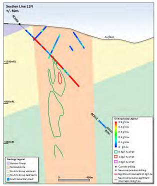
**Figure 17**. Schematic cross section of RC668 and RC659 showing Newcrest and Imperial drill holes and Newcrest drill intercepts (drill intercepts have been reported in Appendix 2 of this report, and in prior Newcrest exploration releases) 0.5g/t AuEq, 1g/t AuEq and 2g/t AuEq shell projections generated from Leapfrog model. Due to window size (+/- 50m) and section orientation (150°) hole may appear on multiple sections.
