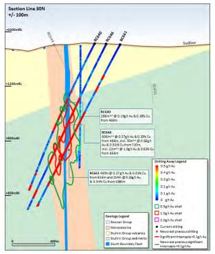
**Figure 26**. Schematic cross section of RC640, RC646 and RC661 showing Newcrest and Imperial drill holes and Newcrest drill intercepts (drill intercepts have been reported in Appendix 2 of this report, and in prior Newcrest exploration releases) 0.5g/t AuEq, 1g/t AuEq and 2g/t AuEq shell projections generated from Leapfrog model. Due to window size (+/- 100m) and section orientation (150°) hole may appear on multiple sections.
