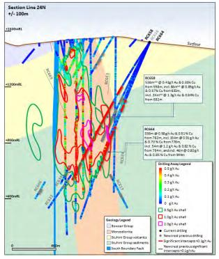
**Figure 25.** Schematic cross section of RC658 and RC664 showing Newcrest and Imperial drill holes and Newcrest drill intercepts (drill intercepts have been reported in Appendix 2 of this report, and in prior Newcrest exploration releases) 0.5g/t AuEq, 1g/t AuEq and 2g/t AuEq shell projections generated from Leapfrog model. Due to window size (+/- 50m) and section orientation (150°) hole may appear on multiple sections.
