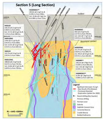
Figure 9. Schematic cross section of geology and significant new drillhole intercepts (looking southwest, Section Line 5a-5b, +/-150m section width, as shown in Figure 4).
