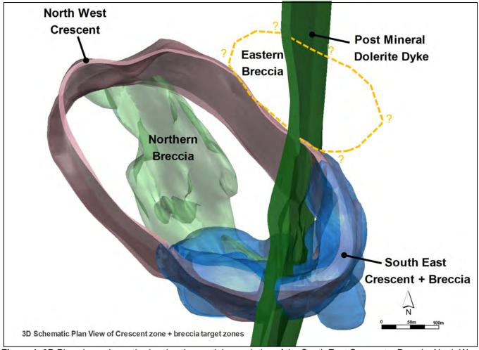
**Figure 1**. 3D Plan view schematic showing the spatial association of the South East Crescent + Breccia, North West Crescent, Northern Breccia and newly recognised Eastern Breccia targets outline projected to surface.
