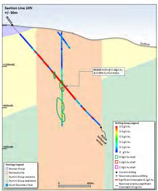
**Figure 16**. Schematic cross section of RC659 showing Newcrest and Imperial drill holes and Newcrest drill intercepts (drill intercepts have been reported in Appendix 2 of this report, and in prior Newcrest exploration releases) 0.5g/t AuEq, 1g/t AuEq and 2g/t AuEq shell projections generated from Leapfrog model. Due to window size (+/- 50m) and section orientation (150°) hole may appear on multiple sections.
