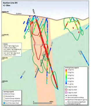
**Figure 13**. Schematic cross section of RC641 showing Newcrest and Imperial drill holes and Newcrest intercepts (drill intercepts have been reported in Appendix 2 of this report, and in prior Newcrest exploration releases) 0.5 g/t AuEq, 1g/t AuEq and 2g/t AuEq shell projections generated from Leapfrog model. Due to window size (+/- 50m) and section orientation (150°) hole may appear on multiple sections.
