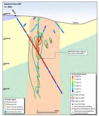
**Figure 18.** Schematic cross section of RC672 showing Newcrest and Imperial drill holes and Newcrest drill intercepts (drill intercepts have been reported in Appendix 2 of this report, and in prior Newcrest exploration releases) 0.5g/t AuEq, 1g/t AuEq and 2g/t AuEq shell projections generated from Leapfrog model. Due to window size (+/- 50m) and section orientation (150°) hole may appear on multiple sections.
