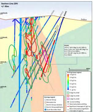
**Figure 23.** Schematic cross section of RC639 and RC647 showing Newcrest and Imperial drill holes and Newcrest drill intercepts (drill intercepts have been reported in Appendix 2 of this report, and in prior Newcrest exploration releases) 0.5g/t AuEq, 1g/t AuEq and 2g/t AuEq shell projections generated from Leapfrog model. Due to window size (+/- 100m) and section orientation (150°) hole may appear on multiple sections.
