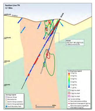
**Figure 15**. Schematic cross section of RC648 showing Newcrest and Imperial drill holes and Newcrest drill intercepts (drill intercepts have been reported in Appendix 2 of this report, and in prior Newcrest exploration releases) 0.5g/t AuEq, 1g/t AuEq and 2g/t AuEq shell projections generated from Leapfrog model. Due to window size (+/- 50m) and section orientation (150°) hole may appear on multiple sections.
