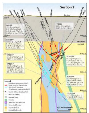
Figure 6. Schematic cross section of geology and significant new drillhole intercepts (looking north, Section Line S2a-S2b, +/-100m section width, as shown in Figure 4).
