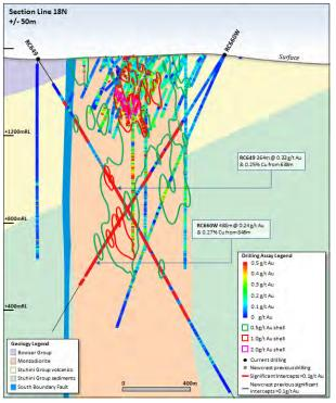
**Figure 22.** Schematic cross section of RC649 and RC660W showing Newcrest and Imperial drill holes and Newcrest drill intercepts (drill intercepts have been reported in Appendix 2 of this report, and in prior Newcrest exploration releases) 0.5g/t AuEq, 1g/t AuEq and 2g/t AuEq shell projections generated from Leapfrog model. Due to window size (+/- 50m) and section orientation (150°) hole may appear on multiple sections.
