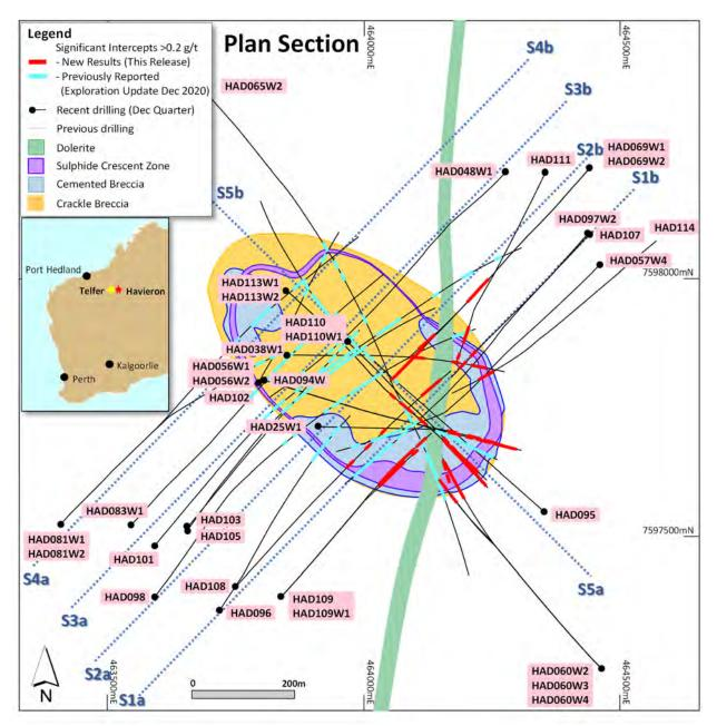
**Figure 4**. Schematic plan view map showing drill hole locations and significant intercepts reported in this release superimposed on the interpreted geology. Existing holes are not shown for the sake of clarity.
