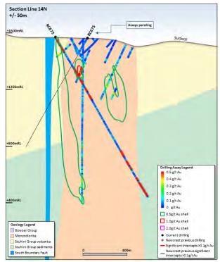
**Figure 20**. Schematic cross section of RC673 and RC675 showing Newcrest and Imperial drill holes and Newcrest drill intercepts (drill intercepts have been reported in Appendix 2 of this report, and in prior Newcrest exploration releases) 0.5g/t AuEq, 1g/t AuEq and 2g/t AuEq shell projections generated from Leapfrog model. Due to window size (+/- 50m) and section orientation (150°) hole may appear on multiple sections.
