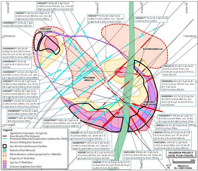
**Figure 2**. Plan view schematic of a horizontal slice at 4700mRL through the Crescent Sulphide Zone and Brecciahosted Zones, showing the extents of the 0.5 and 1.0 g/t Au Leapfrog<sup>TM</sup> grade shells with highlighted newly reported intercepts for the Quarterly Exploration Report including those released on 10 December 2020. Also shown is the Northern Breccia 1 g/t Au Leapfrog shell projected from 4400mRL - drilling is ongoing to confirm the extent of the Northern Breccia.
