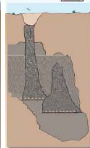
2012 onwards Cadia East Large caving operation
