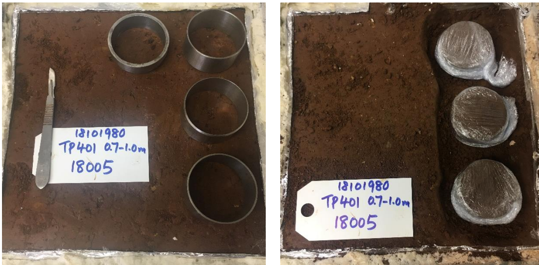
Figure 5: Cored specimens: before coring (left) and after coring (right)
