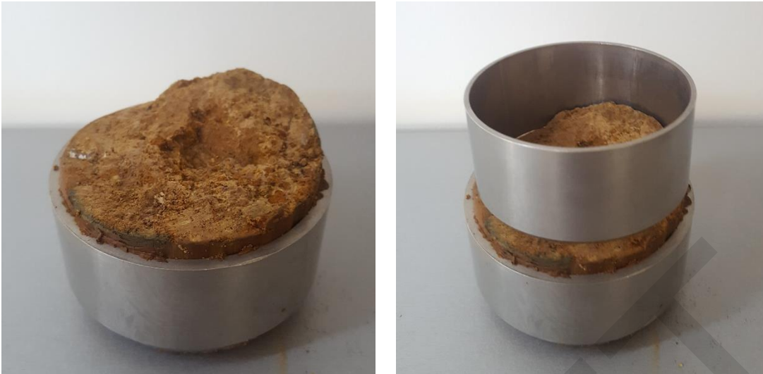
Figure 2: Trimming specimen extruded from 63 mm diameter tube sample to 60 mm diameter
