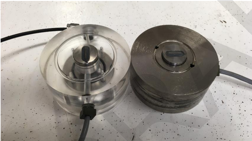
Figure 3: Set of caps with bender elements
