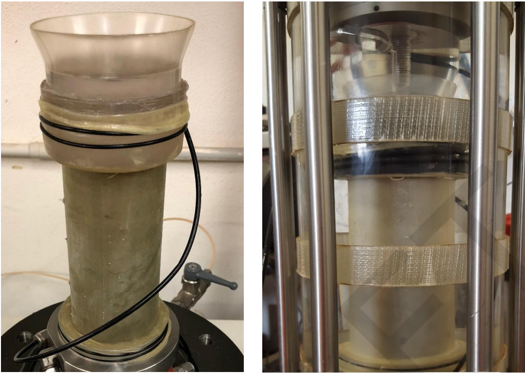
Figure 11: Specimen with suction top cap assembled and inside cell
