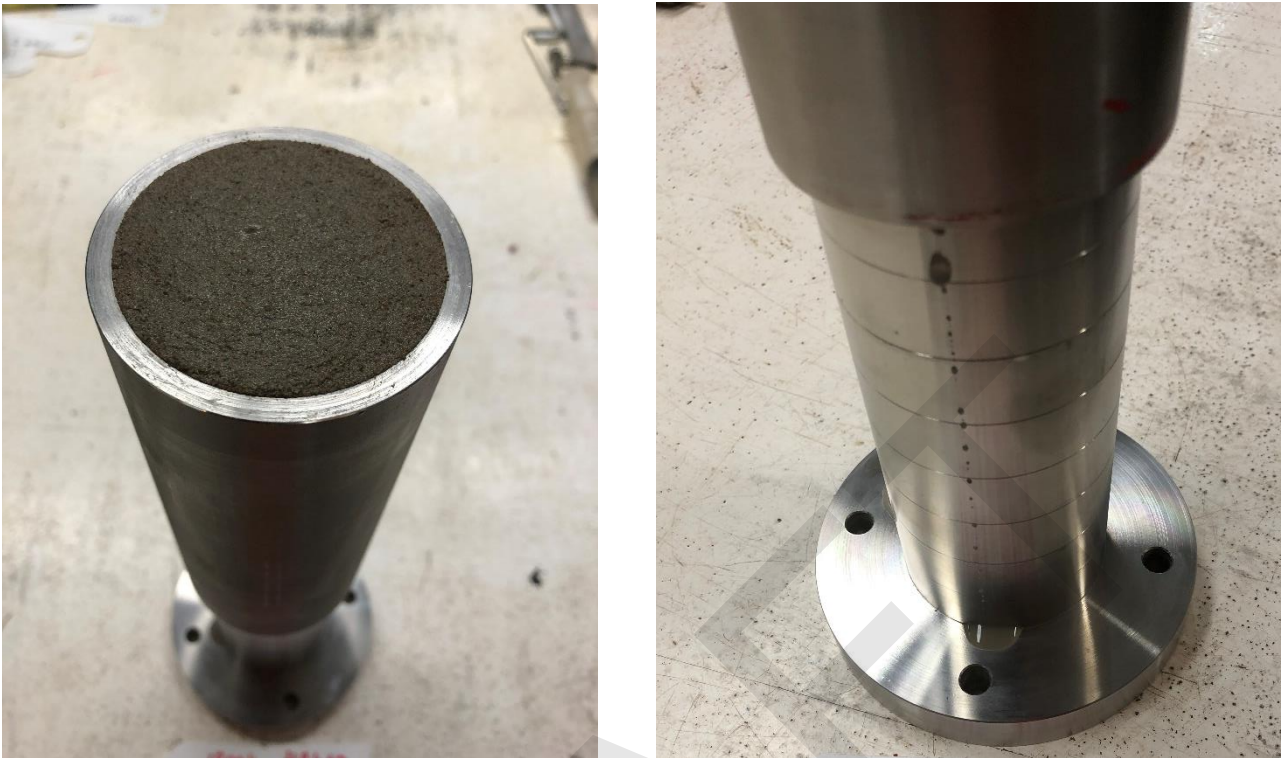
Figure 9: Specimen on top of tamper during water draining stage (left) and water draining from specimen (right)
