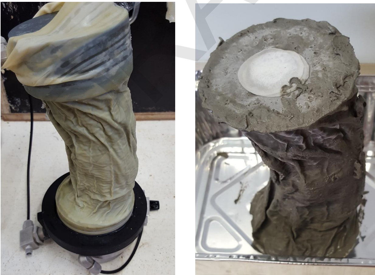
Figure 3: Frozen specimen before removal of membrane and caps (left) and after (right)
