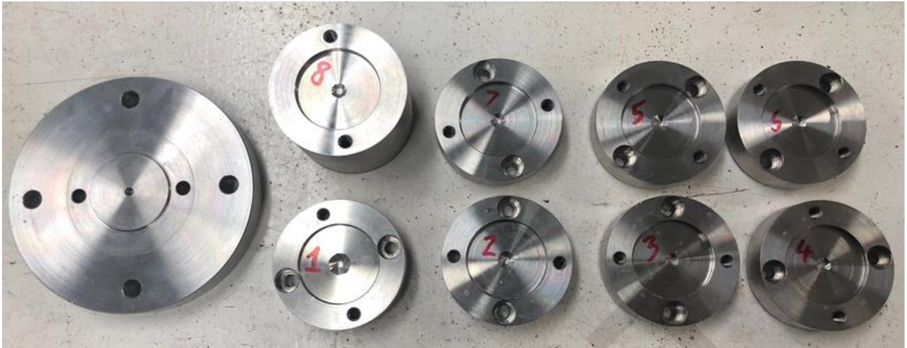
Figure 5: Tamper dismantled with various spacers
