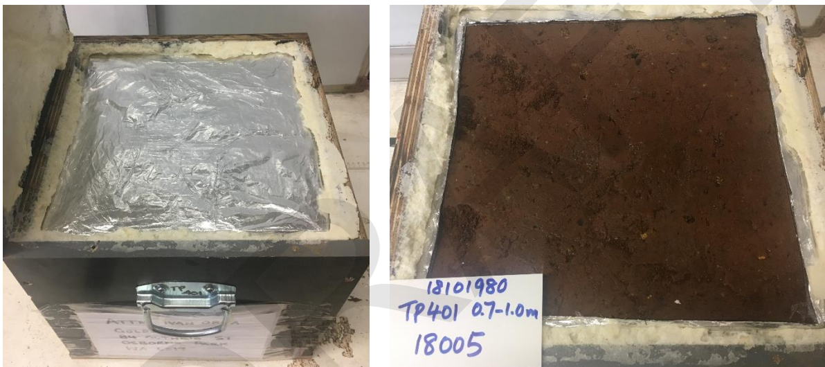
Figure 3: Accessing block sample from the top of box
