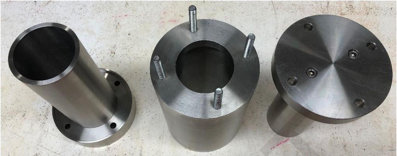
Figure 2: View of different components of compactor: mould base platen with the inner sleeve (left), outer sleeve (middle) and adjustable height tamper with top platen to allow controlling the height (right)
