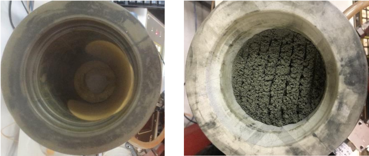
Figure 6: Split moulds with membrane under suction (left) and during specimen preparation with scarified layer prior tamping of next layer (right)
