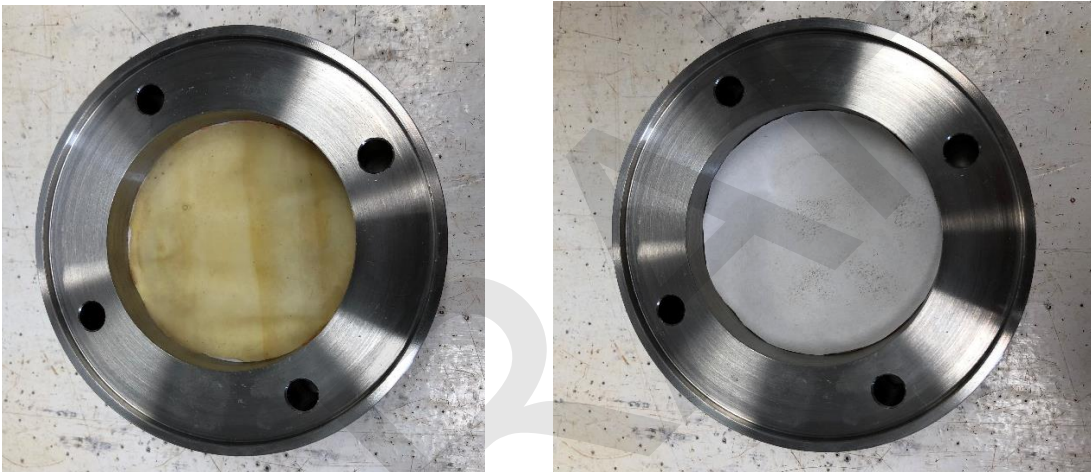
Figure 3: Mould base platen with sandwich of paper filter, latex membrane and paper filter at its bottom
