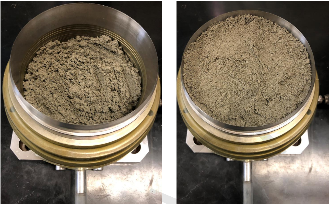
Figure 2: Placement of loose sample in DSS mould with stainless steel ring used to facilitate material placement
