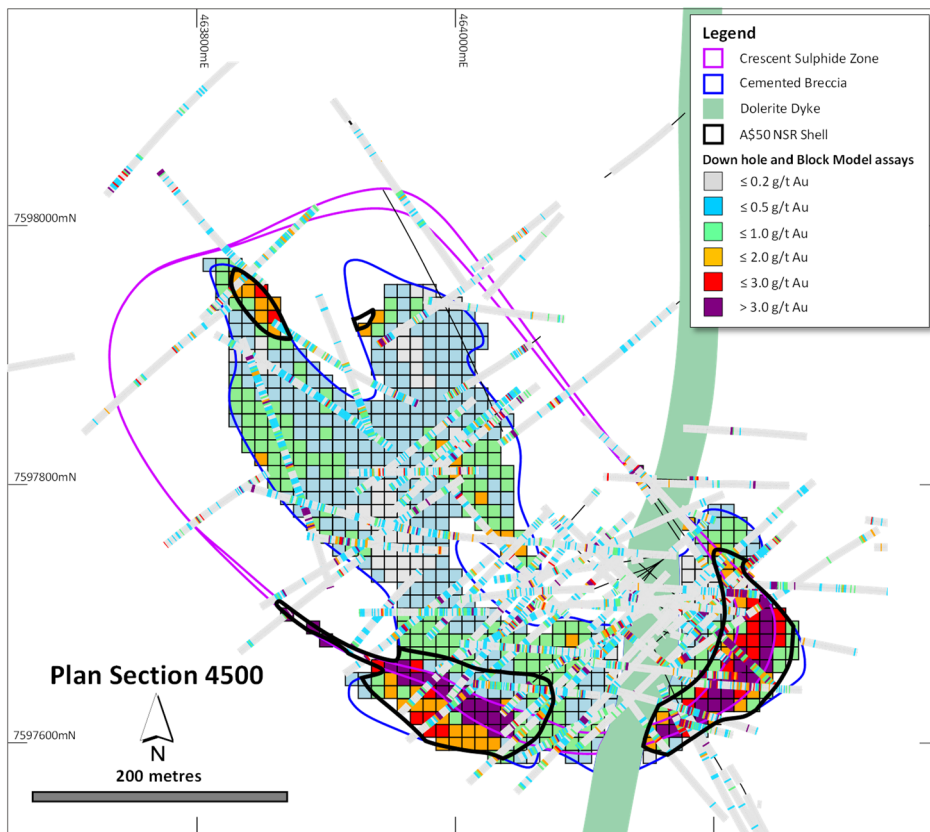
Figure 3. Plan view schematic of a horizontal slice at 4500mRL with 50m section width through the Crescent Sulphide Zone and breccia-hosted mineralisation, showing the block model and 2m downhole composites coloured by gold grade in relation to the A$50/t NSR breakeven constraining shell. Also shown is the Crescent Zone, Cemented Breccia and Dolerite Dyke outlines.
