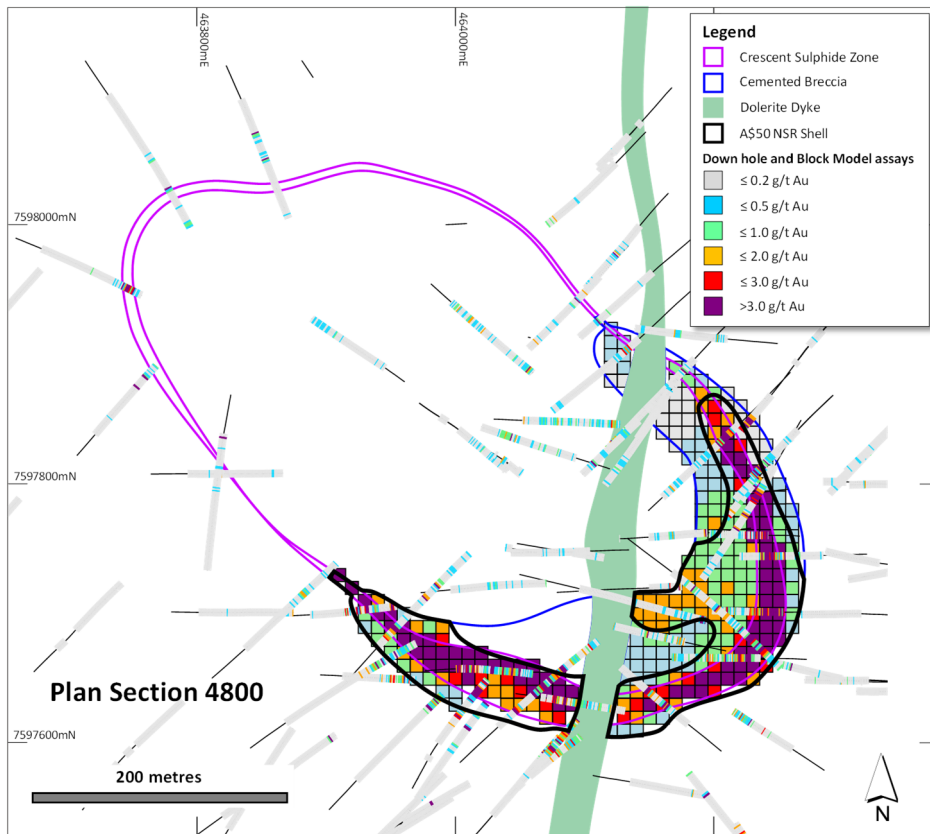
Figure 2. Plan view schematic of a horizontal slice at 4800mRL with 50m section width through the Crescent Sulphide Zone and breccia-hosted mineralisation, showing the block model and 2m downhole composites coloured by gold grade in relation to the A$50/t NSR breakeven constraining shell. Also shown is the Crescent Zone, Cemented Breccia and Dolerite Dyke outlines.
