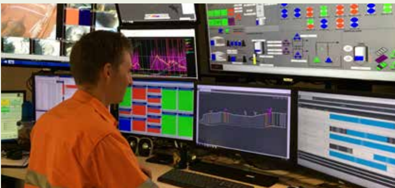
Telfer Underground Mine Control Supervisor Brad Brown uses “Dingo” to assist in allocating trucks and loaders to optimal locations in Telfer’s sub-level cave mine.
